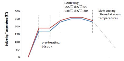
Reflow soldering method:
