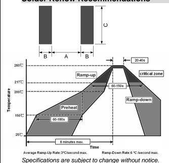
• If reflow temperatures exceed the recommended profile, devices may not meet the performance requirements. • Devices are not designed to be wave soldered to the bottom side
