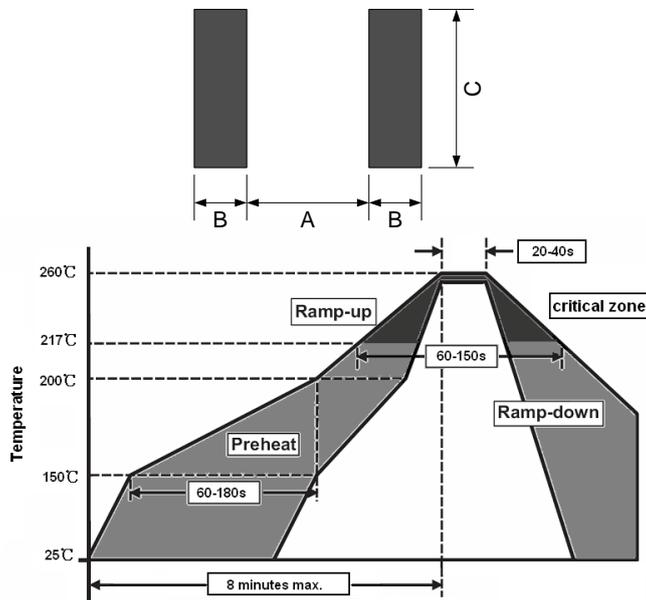
Average Ramp-Up Rate: 3°C/second max. Ramp-Down Rate: 6 °C /second max.
